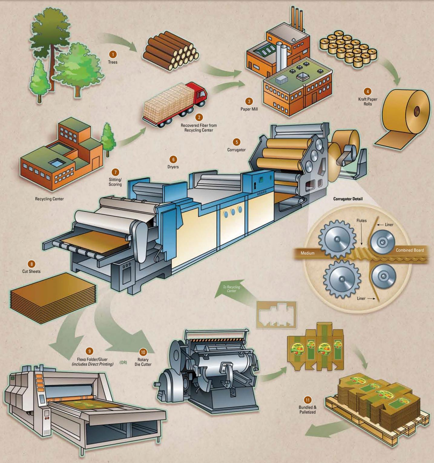
The production of corrugated boxes begins much like any other paper product. Wood (1) from trees harvested from responsibly managed forests and fiber (2) recovered from paper recycling centers are processed into pulp and made into paper at a paper mill (3). In this process, two different types of brown paper (kraft) are produced:
